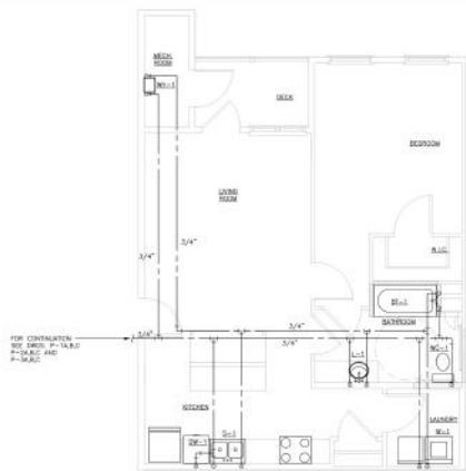
PLUMBING ENLARGED UNIT PLAN A-1A HC SCALE: 1/4" = 1'-0"
